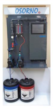
Chlorine dioxide is typically produced on site with a generator such as the one pictured here.
